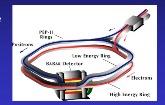
Electrons & positrons are accelerated to their final energies in a linear accelerator and then "injected" into the PEP-II storage rings:
